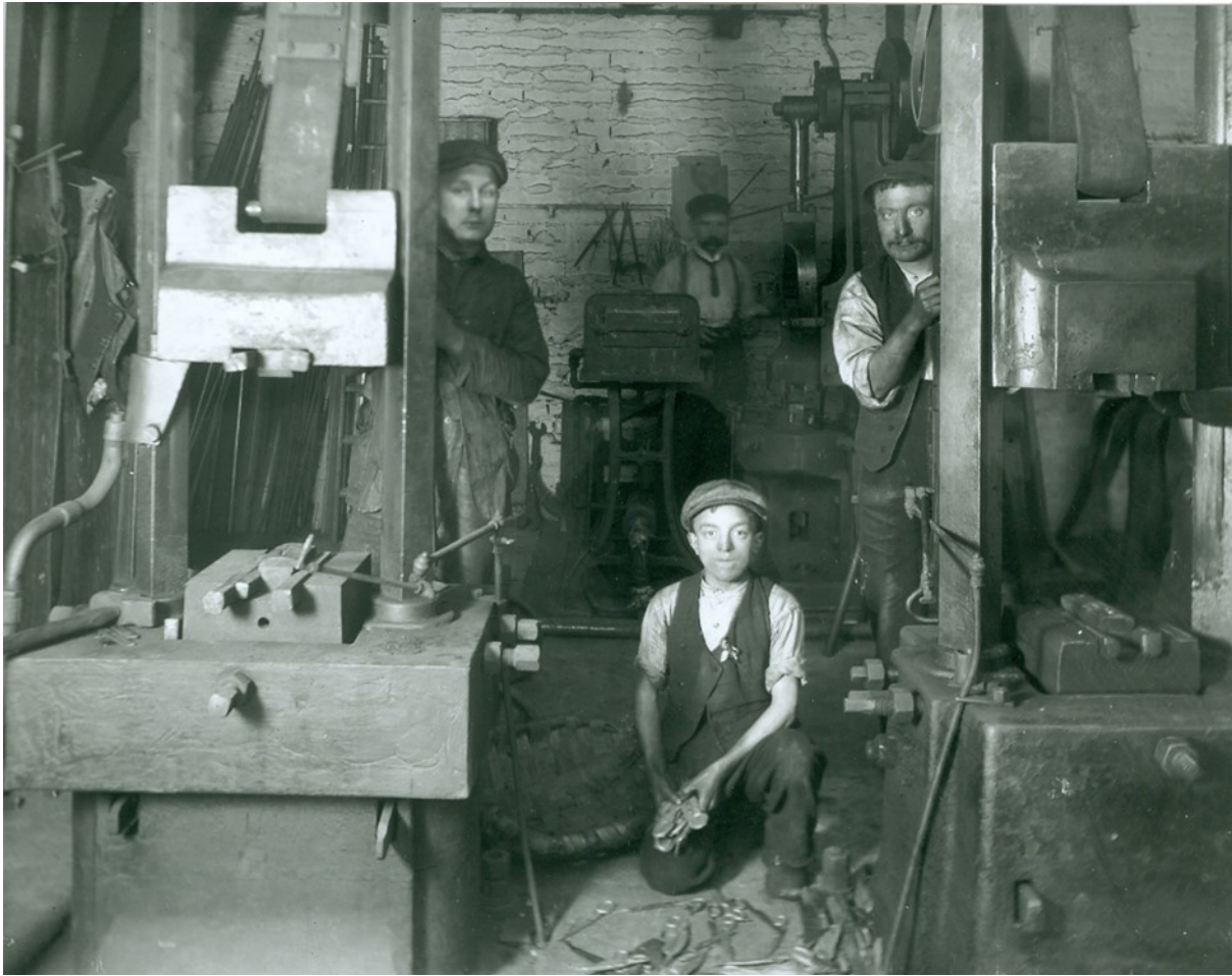
Drop stamping at Eye Witness cutlery works, 1910 - PH.CUT.229
