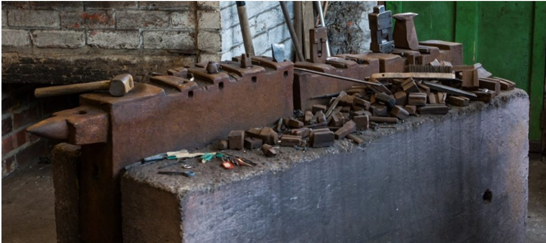
Forging anvils and dies in Peter Goss's workshop at Kelham Island Museum
