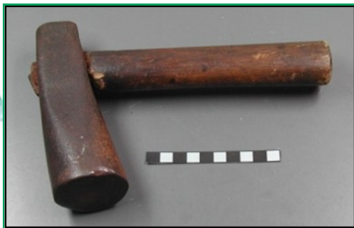
File forging hammer; boss for forming a three square file blank; a flat and a three square file blank
