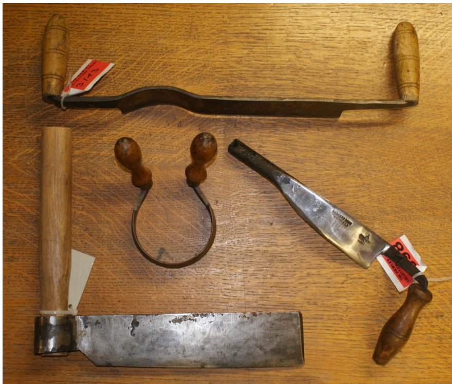
Coopers' tools from the Hawley Collection (L to R) Top: reverse two-handed crumming knife Bottom: axe, roundshave, crumming knife
